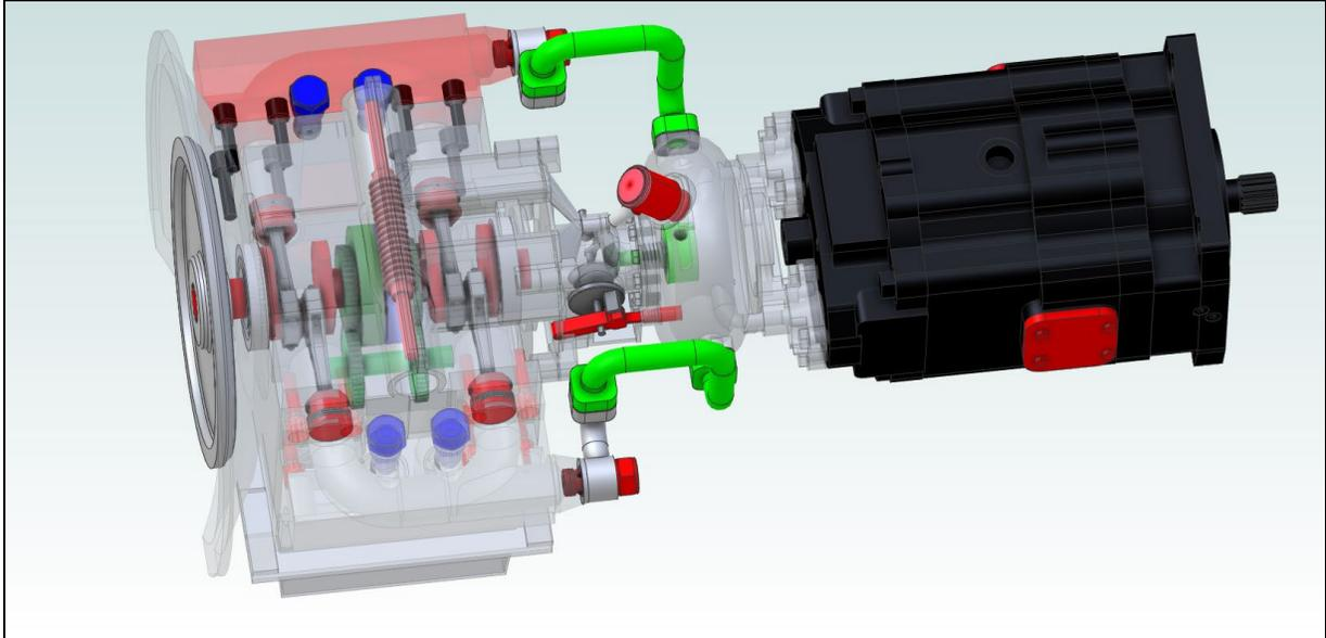
*AMT Controlled VDS with paired pistons at 0° in-phase relationship, with maximum displacement*
