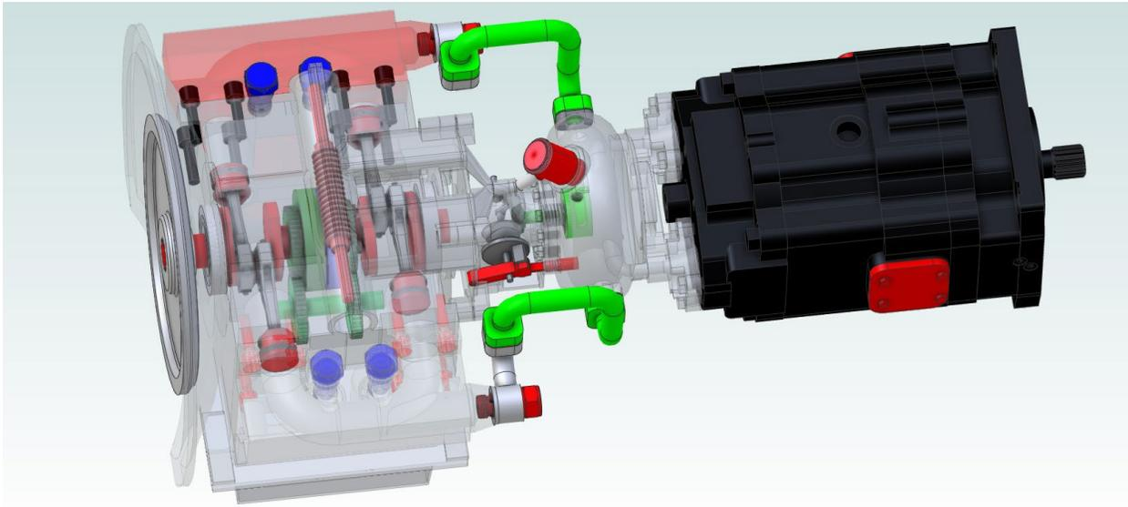
*AMT Controlled VDS with paired pistons at 180° out-of-phase relationship, with zero displacement*
